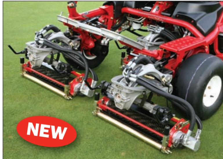
The new Toro TriFlex does not have grass box carrier frames like previous models did (right). This enables clear access for changing cassettes with the units still on the mower - even the centre unit!
